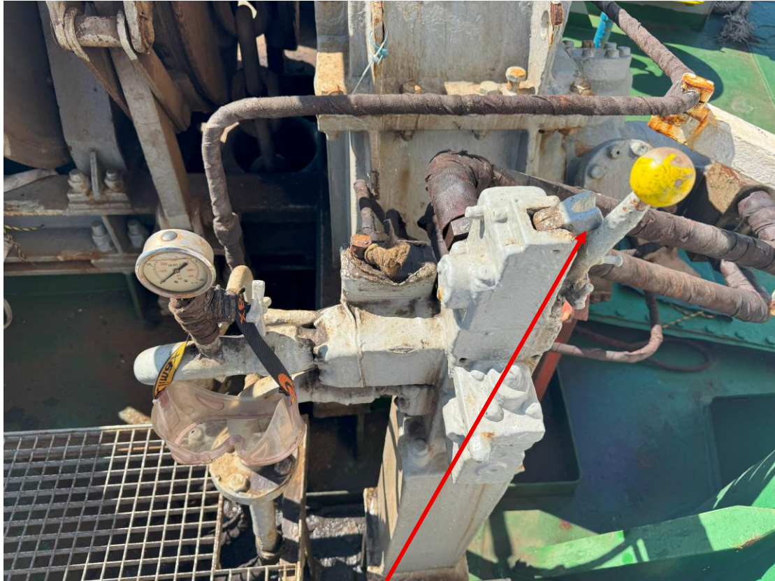
Fig15- View of lever held in position by safety catch
