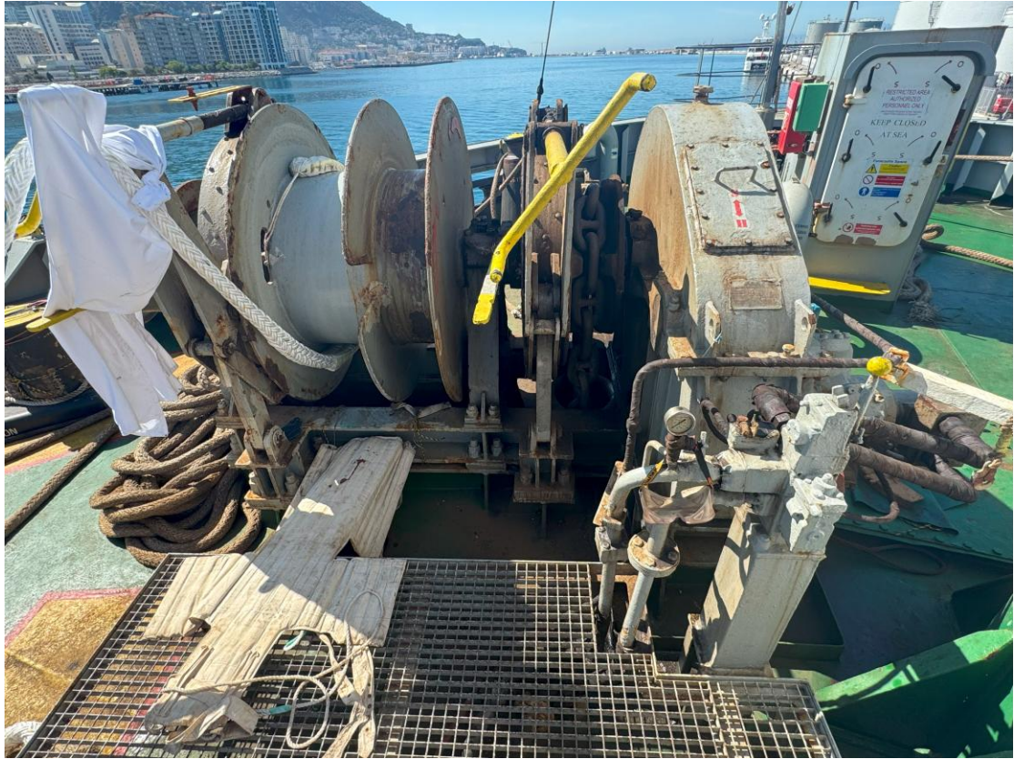
Fig 8 – View of Winch leading fwd
